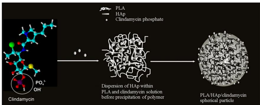
**Fig. 1** Proposed mechanism for the formation of spherical PLA/HAp loaded with clindamycin phosphate (Adapted from Vukomanović et al. [9])
